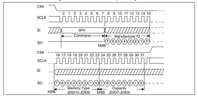
Figure 28. Read Identification ID Sequence Diagram
