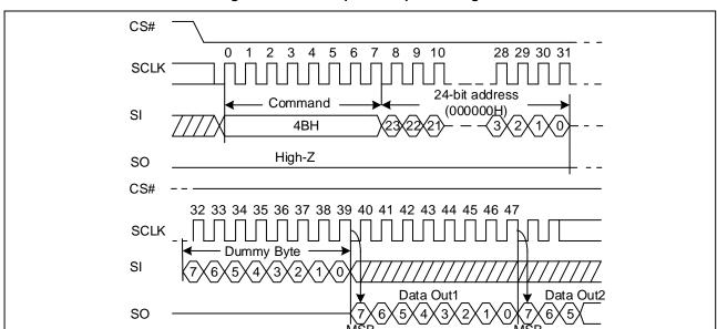
Figure 36. Read Unique ID Sequence Diagram
