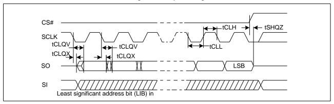
Figure 43. Resume to Suspend Timing Diagram
