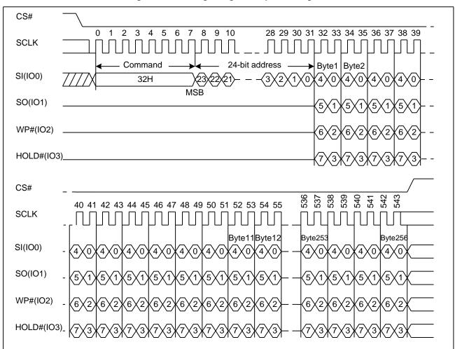
Figure 19. Quad Page Program Sequence Diagram
