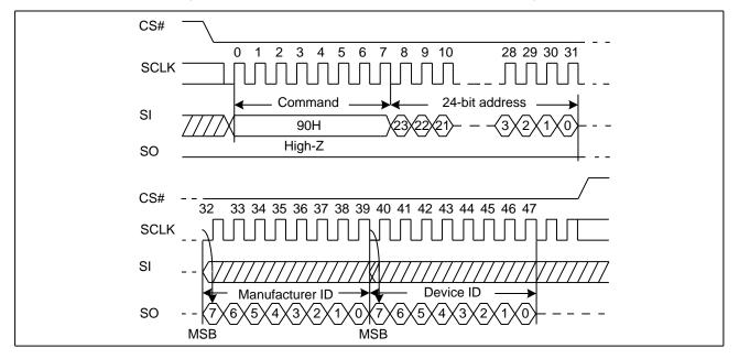
Figure 27. Read Manufacture ID/ Device ID Sequence Diagram
