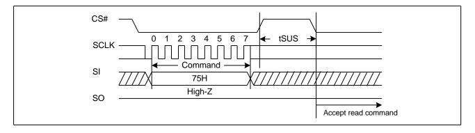
Figure 30. Program/Erase Suspend Sequence Diagram
