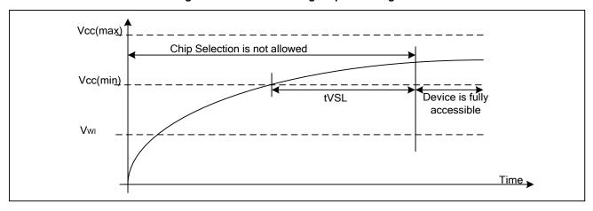
Table6. Power-Up Timing and Write Inhibit Threshold
