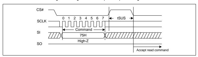
Figure 29. Program/Erase Suspend Sequence Diagram
