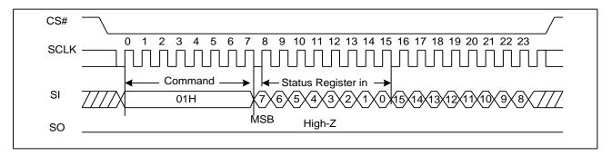
Figure 5. Write Status Register Sequence Diagram
