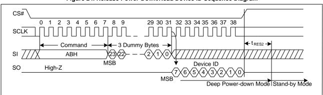
Figure 24. Release Power-Down/Read Device ID Sequence Diagram
