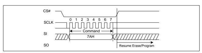
Figure 30. Program/Erase Resume Sequence Diagram
