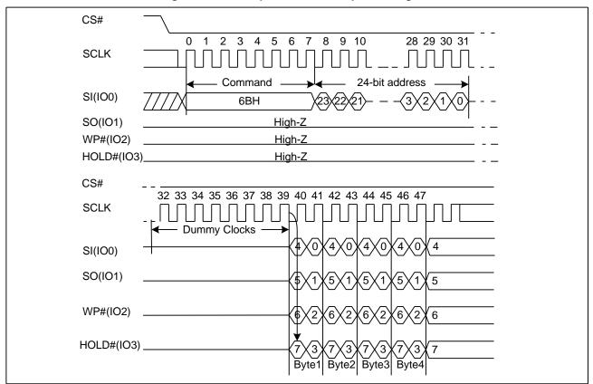
Figure 8. Quad Output Fast Read Sequence Diagram
