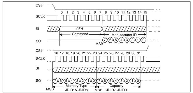
Figure 26. Read Identification ID Sequence Diagram
