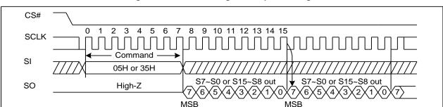
Figure 4. Read Status Register Sequence Diagram
