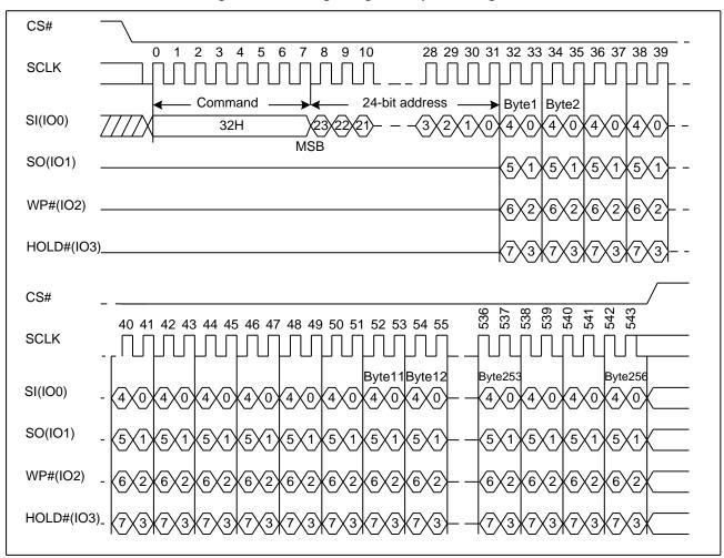
Figure 17. Quad Page Program Sequence Diagram
