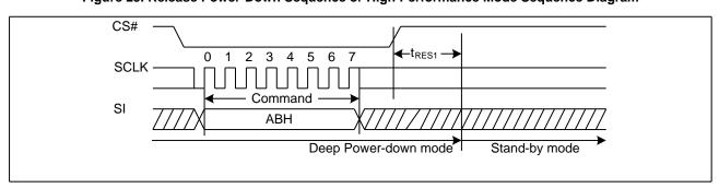
Figure 23. Release Power-Down Sequence or High Performance Mode Sequence Diagram
