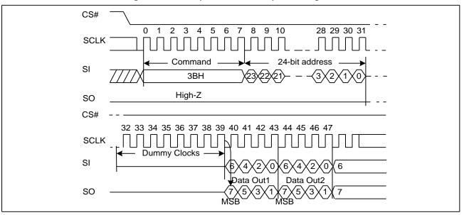
Figure 7. Dual Output Fast Read Sequence Diagram
