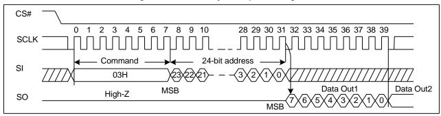
Figure 7. Read Data Bytes Sequence Diagram
