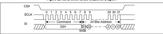
Figure 22. 32KB Block Erase Sequence Diagram
