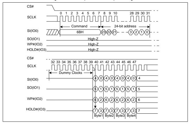
Figure 10. Quad Output Fast Read Sequence Diagram
