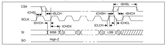
Figure 44. Output Timing
