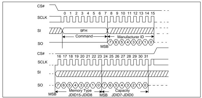
Figure 31. Read Identification ID Sequence Diagram
