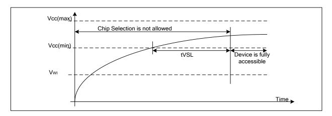
Table6. Power-Up Timing and Write Inhibit Threshold
