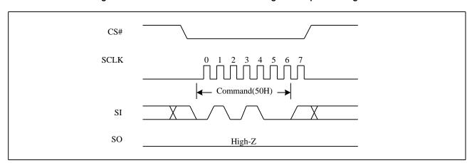
Figure 4. Write Enable for Volatile Status Register Sequence Diagram
