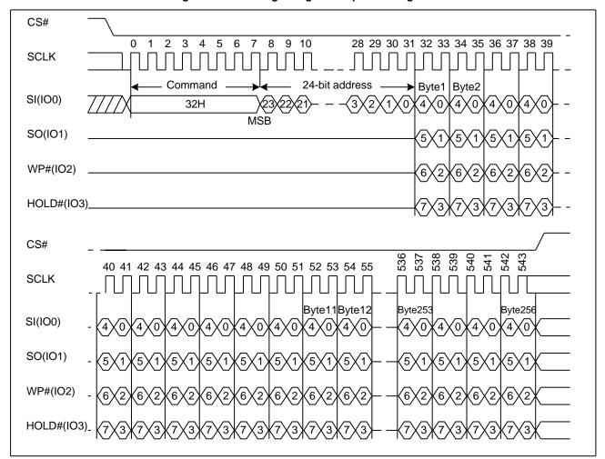
Figure 19. Quad Page Program Sequence Diagram
