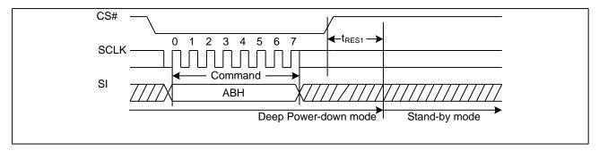
Figure 27. Release Power-Down/Read Device ID Sequence Diagram
