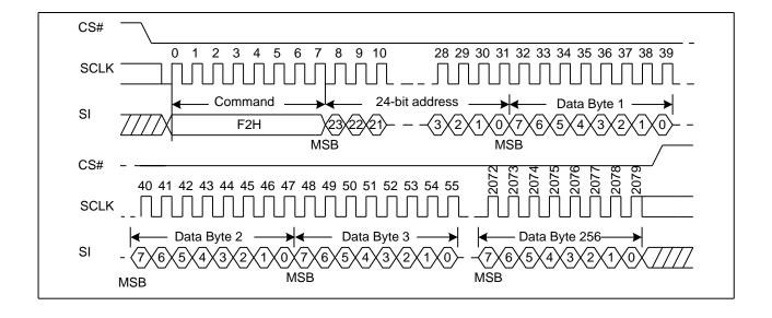
Figure 20. Fast Page Program Sequence Diagram
