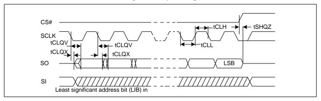
Figure 45. Resume to Suspend Timing Diagram
