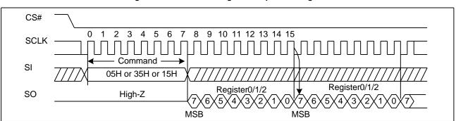
Figure 5. Read Status Register Sequence Diagram
