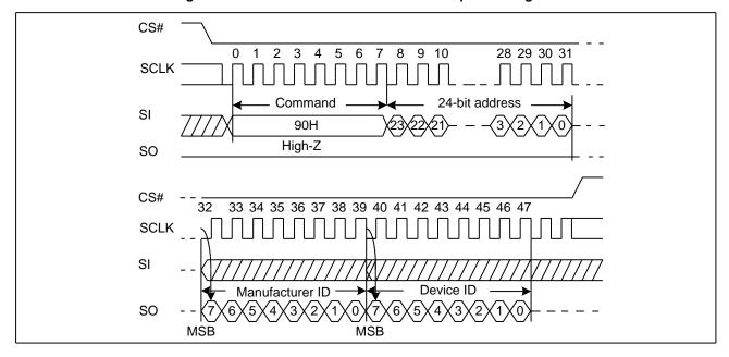
Figure 28. Read Manufacture ID/ Device ID Sequence Diagram
