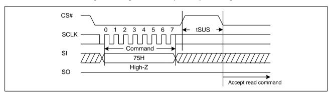
Figure 34. Program/Erase Suspend Sequence Diagram
