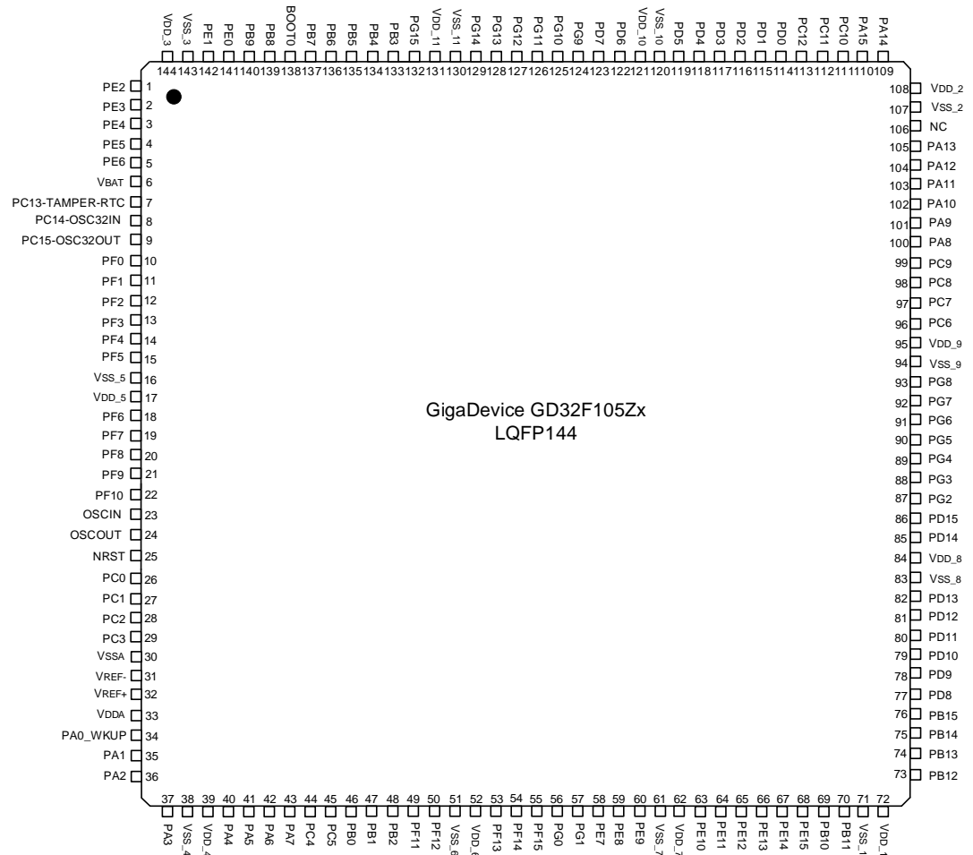
Figure 2-2. GD32F105Zx LQFP144 pinouts
