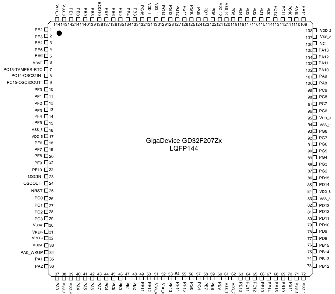
Figure 2-3. GD32F207Zx LQFP144 pinouts
