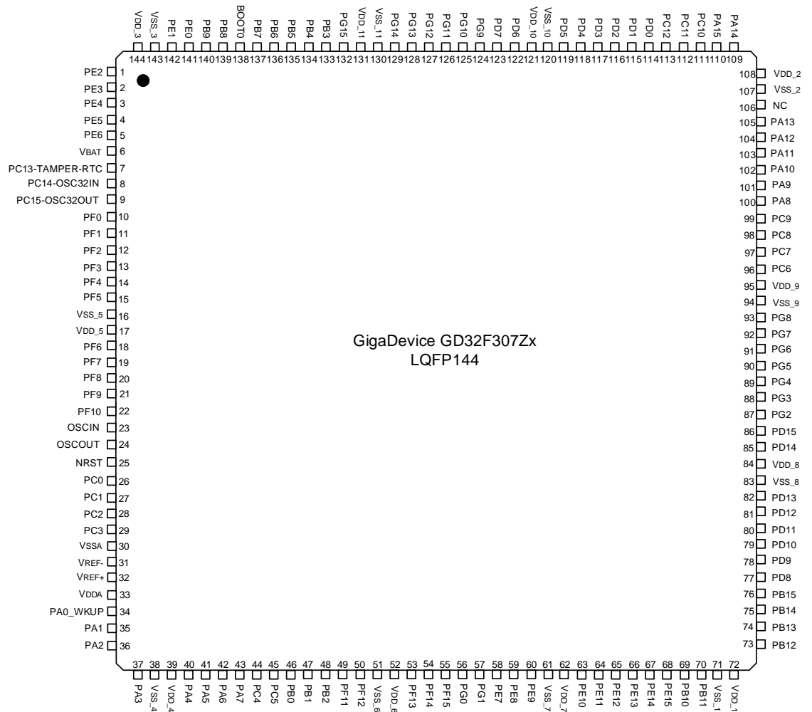
Figure 2-2 GD32F307Zx LQFP144 pinouts
