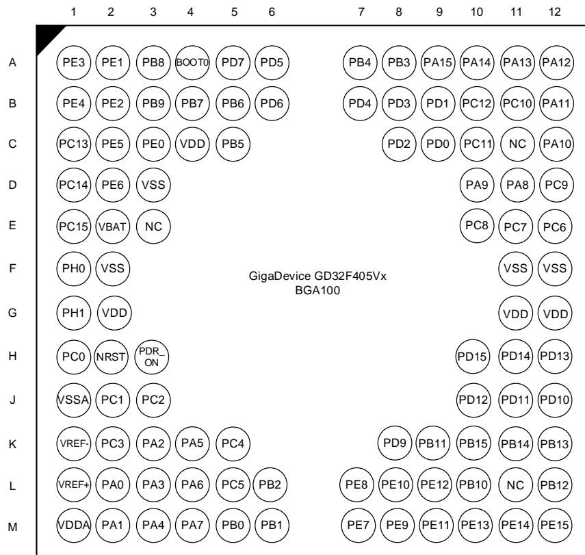
Figure 2. GD32F405Vx BGA100 pinouts
