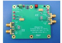
The 050-301-EVALBOARD (Size #8 evaluation board) can be used in one of three test configurations to test active size #8 opto-electronic contacts (i.e. p/n 050-301, 050-307, 050-367, and other general size #8 contacts). The options are:
