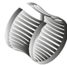
Figure 2. Conventional Contact on the left, LouverBand Contact on the right
