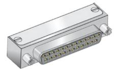
Low profile right angle PC tail HiPer-D socket connectors feature rugged machined aluminum shell and stainless steel cover for improved EMI protection. Contacts are non-removable size, #20 or #22. Intermateable with standard M24308-type D-Subminiature connectors, the HiPer-D features epoxy potting for environmental sealing. Threaded holes on the rear of the connector allow attachment to circuit board. Glass-reinforced thermoset epoxy insulators. 1000 VAC, 5 Amps (#22) or 7.5 Amps (#20).
