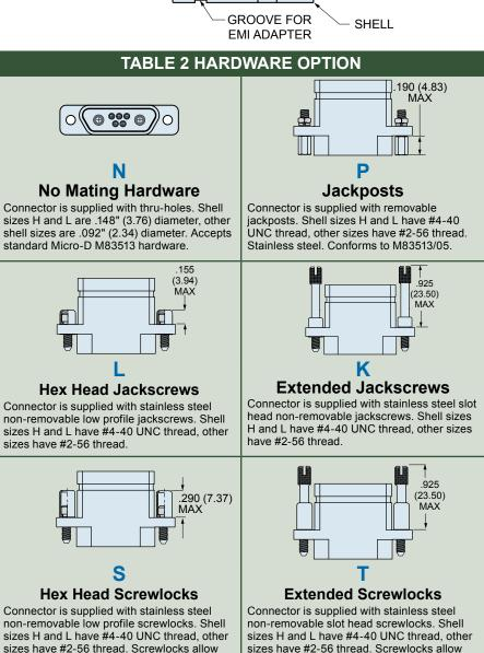
the connector to be mated before the screws
