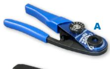
These crimp tools perform precision eight indent crimps for gas tight wire terminations and excellent tensile strength. Adjustment wheel has 8 settings. Ratchet mechanism prevents improper crimps. Use with bayonet type positioners. Check calibration with M22520/3 gages. Length is 6.75 inches, weight is approx. 10 oz.
