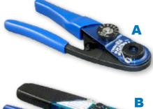
These crimp tools perform precision eight indent crimps for gas tight wire terminations and excellent tensile strength. Adjustment wheel has 8 settings. Ratchet mechanism prevents improper crimps. Use with bayonet type positioners. Check calibration with M22520/3 gages. Length is 6.75 inches, weight is approx. 10 oz.
