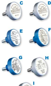
These bayonet-type positioners hold contacts at correct height for crimping with M22520/2 type miniature step adjustable tools, above. Face plate shows correct tool settings.
