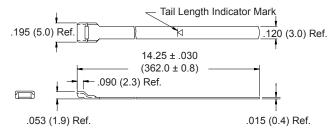
**The 600-052 Standard Band** is precision constructed of 300 Series SST/Passivate I.A.W AMS 2700 and designed for use with the 600-058 Hand Banding Tool or the 600-067 Pneumatic Banding Tool. Double-wrapped bands will accommodate diameters up to approximately 1.8 inches (45.7). Bands may be ordered flat (600-052) or precoiled (600-052-1). Bands come bagged and tagged in quantities from 1 to 100. **Reference:** *BAND-IT*<sup>®</sup> **part number A10086**
