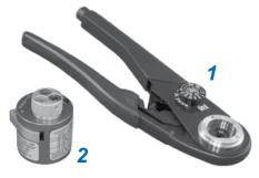
Crimp tool for use with size #16 and #12 power pins. 9.75 inches OAL, 1.25 pounds. Use with M39029/57 and /58 contacts and 809-093 adapters.
