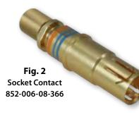
Coax contacts accept M17/095-RG180 cable. These snap-in, rear release contacts fit Glenair Series 80 Mighty Mouse connectors and Glenair MIL-DTL-38999 Series I, III and IV connectors with size #8 cavities. Crimp termination. Gold-plated copper alloy, Teflon insulator. Supplied unassembled. Order sealing boot separately (fig. 3). 1 A current rating, 500 Vac. SAE AS39029 gualified.
