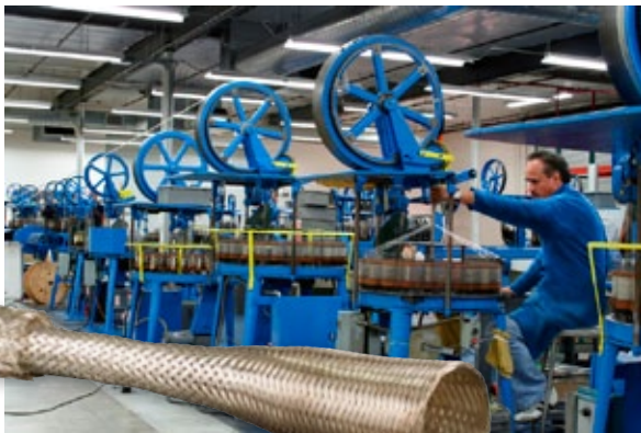
Glenair operates one of the largest multi-spindle overbraiding operations in the world
