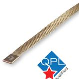
Glenair MIL-DTL-24749 Rev B Type IV ground straps solve harsh-environment shipboard corrosion and electrical resistance problems with a unique 50% Stainless Steel 316L / 50% Nickel 200 36AWG blend braid, and passivated Stainless Steel lugs. These US Navy-approved ground straps are qualified to the rigorous standards of M24749, and are tested beyond the mil-spec to survive 1000 hours salt spray. Allowed usages for Type IV straps can be found in MIL-STD-1310H.
