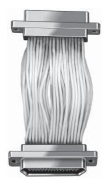
Micro-D Connectors are available as back-toback complete assemblies. These cables can be used as connector savers or gender changers. These assemblies are wired pointto-point (contact 1 to contact 1, etc.).
