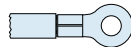
Lug Terminal for Attaching Receptacle Covers to a Panel with a Screw
