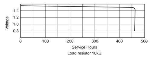
Average Service Capacity: 70 mAh (rated capacity at  $10k\Omega$  load, cut off voltage 1.2V at  $20^{\circ}C$ )
