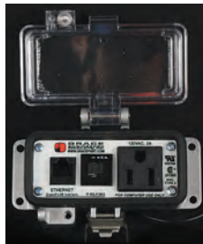
P-R2-F3R3 (1) Ethernet (RJ45), 3 amp CB, in a UL Type 4 Housing, with Simplex Outlet
