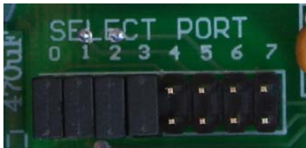
FIG 3: Port driver selection jumpers
