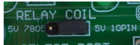
FIG1: Power selection jumpers
