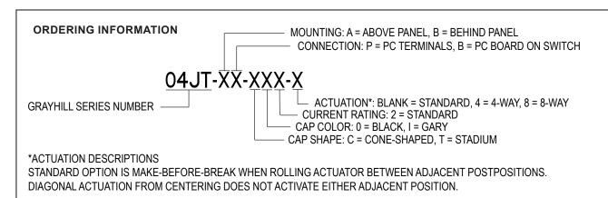
4-WAY OPTION IS BREAK-BEFORE-MAKE PREVENTING ADJACENT POSITIONS FROM BEING ACTIVE SIMULTANEOUSLY. DIAGONAL ACTUATION FROM CENTER DOES NOT ACTIVATE EITHER ADJACENT POSITION.
