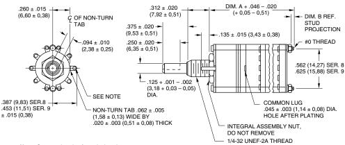
Note: Common location for a single pole per deck switch. For common location on multi-pole switches, see circuit diagrams.
