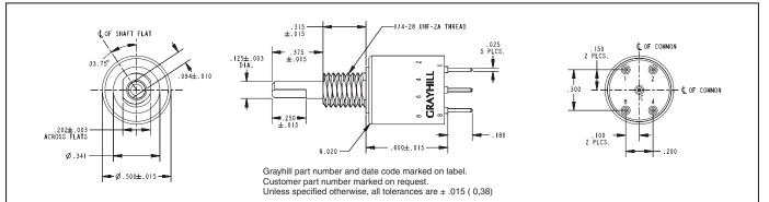
Rated: 25,000 cycles with logic compatible loads. Make and break 200 mA. Contact Resistance: 500 milliohms maximum (less than 100 milliohms initially) Insulation Resistance: 1000 megohms minimum (10,000 megohms initially) Dielectric Strength: 250 Vac minimum
