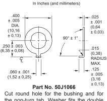
Cut round hole for the bushing and for the non-turn tab. Washer fits the double D bushing flats. Washer is sold only when accompanied by an order for a like number of switches. Washer is 302 stainless steel.
