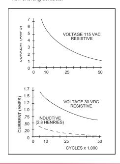
These curves allow you to predict the expected life of the switch once you know the voltage, current and type of load. Also note that each cycle is approximately a 360° rotation and a return. For a ten position switch this would be a rotation from position 1 to position 10 and back to 1. This cycle runs approximately ten times a minute. Thus testing causes more electrical and mechanical wear than what the switch incurs in actual use.
