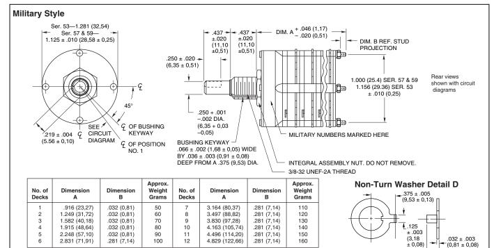
Mounting Hardware: Two mounting nuts, .094" (2,39) thick by .562" (14,27) across flats, one internal tooth lockwasher and one non-turn washer (see detail D for dimensions), are supplied with switch.
