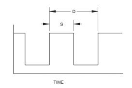
DUTY CYCLE DEFINED AS THE RATIO BETWEEN THE HIGH TIME (S) AND THE PERIOD (D) OF THE PWM SIGNAL AS SHOWN IN FIGURE ABOVE.
