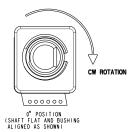
Encoder has ratiometric analog output (output levels are proportional to the supply voltage). Specifications on this datasheet apply @ VDD = 5.00 V.
