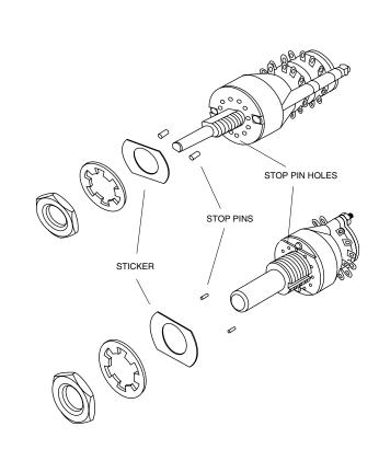
The adjustable stop Series 71 rotary switches allow you to change the number of positions per pole. Simply remove and relocate stop pins in the holes in the front of the switch. The pins are held in place by a self adhesive sticker which fits over the front plate.
