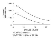
One cycle is 360° rotation and a return through all switch positions to the starting position. The data for the curve was measured at sea level, 25°C and 68% relative humidity with the following limiting criteria:
