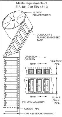
Each reel has a 15.750 inch (390 mm) minimum leader and a 6.30 inch (160 mm) minimum trailer.
