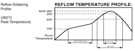
WAVE SOLDERING: 260°C maximum solder temperature for 5 seconds max. \*\* Note: 100% matte tin terminal plating does not meet MIL-S-83504 for lead content. Specifications are subject to change. Please refer to the current datasheet on www.grayhill.com for the most current published specifications for this product.
