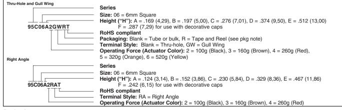
Packaging Thru-Hole: Bulk,1000 pcs/bag. Surface Mount: 77 pcs/tube, 1000 pcs/reel (.169" height), 900 pcs/reel (.197" height), 500 pcs/reel (.276" and .287" height), 380 pcs/reel (.374" height). Right Angle: Bulk, 1000 pcs/bag.
