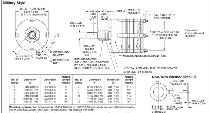
Grayhill part number and date code marked on detent cover label. Customer part number marked on request. Military part number marked when required.
