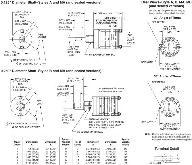
Angle C is 15° in 12 position switches and 36° in 10 position switches
