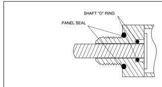
The shaft is sealed by an O-ring inside the bushing. The panel is sealed by an O-ring at the base of the bushing.
