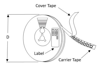
Tape and Reel Packaging with Reel Diameter Noted (D)
