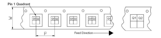
Carrier Tape Width (W), Pitch (P), Feed Direction and Pin 1 Quadrant Information
