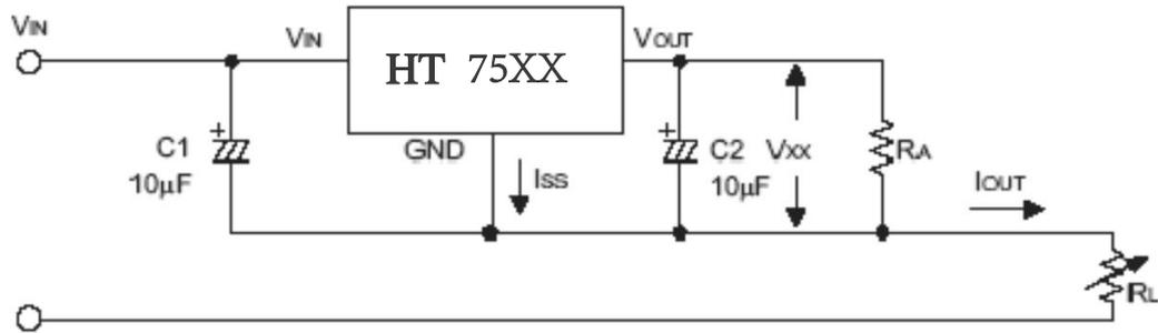
$$I_{OUT} = V_{XX}/R_X + I_{SS}$$
