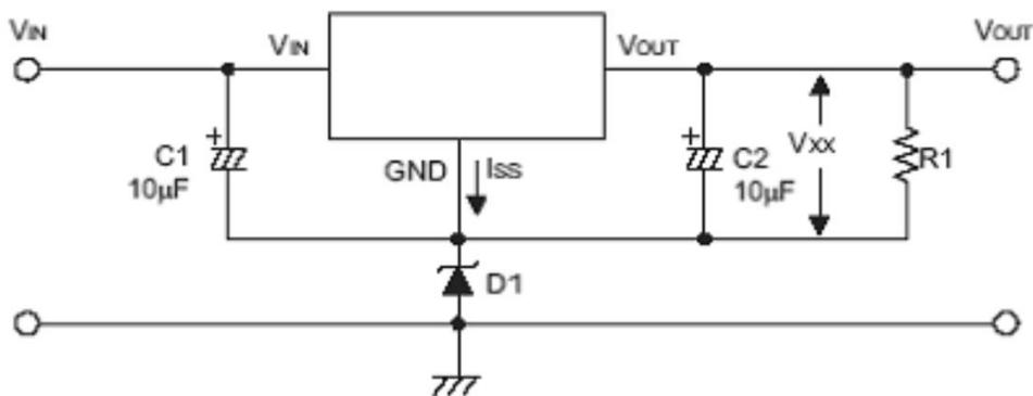
$$V_{OUT} = V_{XX} + VD1$$
