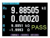
**ENLARGE** Display **Enlarge Measurement Results and** Include PASS/FAIL Judgment
