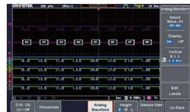
Display analog waveform converted from digital signal
