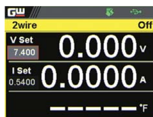
Voltage, Current and Temperature Measurement
