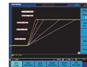
The Adjustable Rise Time of the PSW 800V
