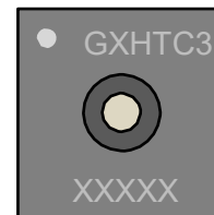
Figure 8 Laser marking on GXHTC3, the top line with the pin-1 indicator and the sensor type, the bottom line with the 5-digit alphanumeric tracking code.
