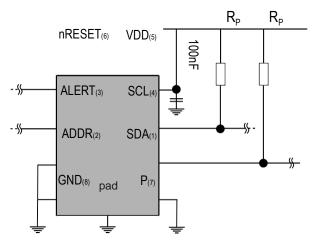
**Figure 4** Typical application circuit. Please note that the positioning of the pins does not reflect the position on the real sensor. This is shown in Table 5.
