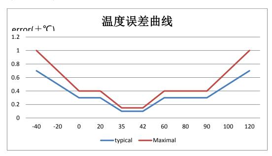
Figure 2 Temperature accuracy of the GXTS03 sensor.
