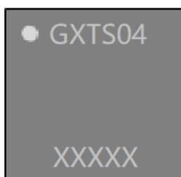
Figure 4 Laser marking on GXTS04, the top line with the pin-1 indicator and the sensor type, the bottom line with the 5-digit alphanumeric tracking code.
