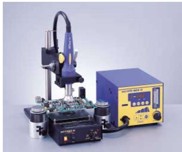
Setting example HAKKO FR-803, HAKKO 853, Rework Fixture, Omnivise
